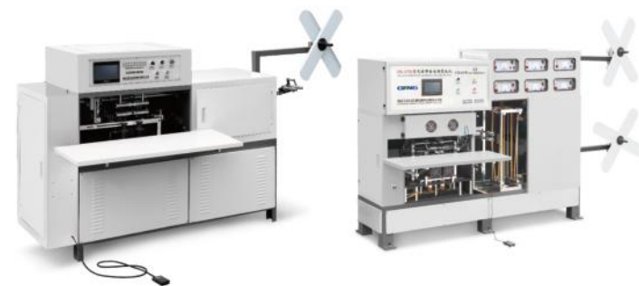
诺15-G/F700 OYANG15-G/F700 自动手提烫把机 Automatic Soft Handle Sealing Machine
